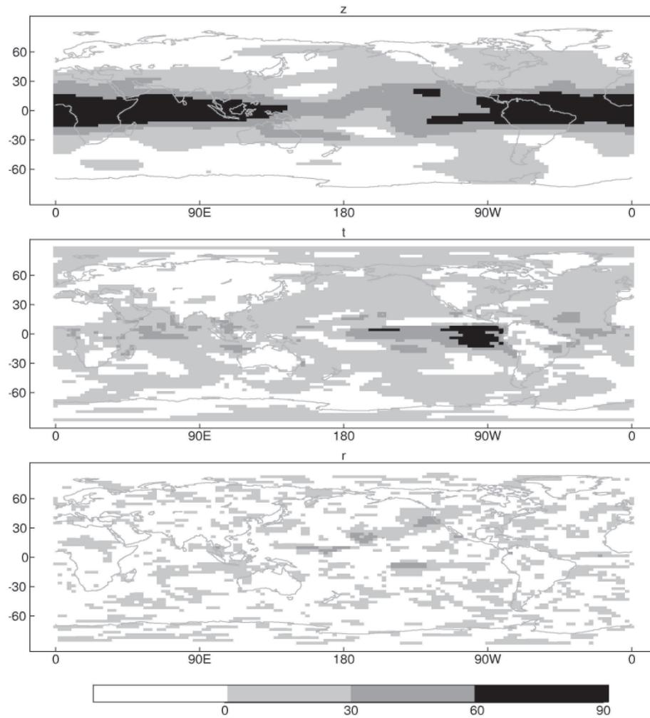
Figure 2. Geographical distribution of skill for model forecasts, with lead 1, of  $z$  (200 hPa height),  $t$  (temperature), and  $r$  (rainfall rate). Unshaded regions are those with negative skill.
