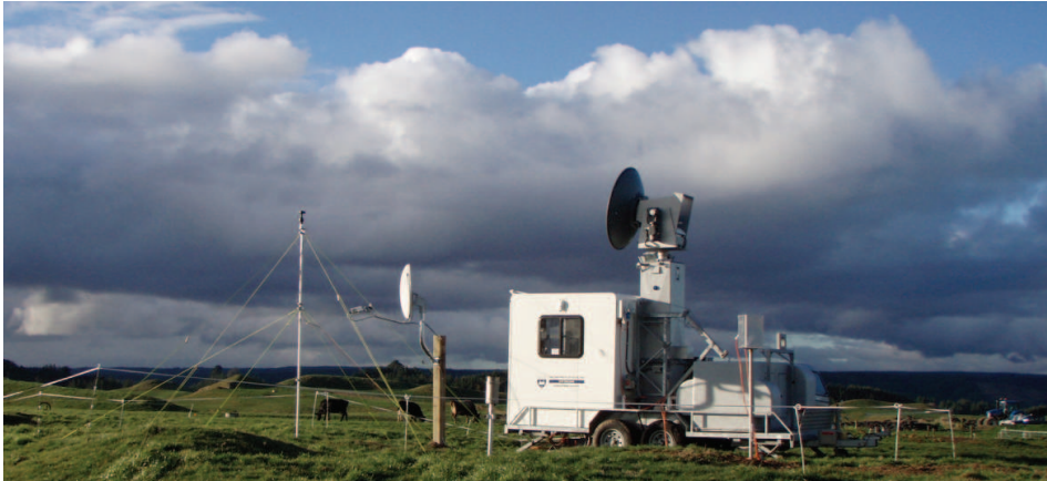
Figure 1: The Trailer Radar deployed in a field. Ancillary equipment in view includes an anemometer, drop counting rain gauge and satellite dish.
