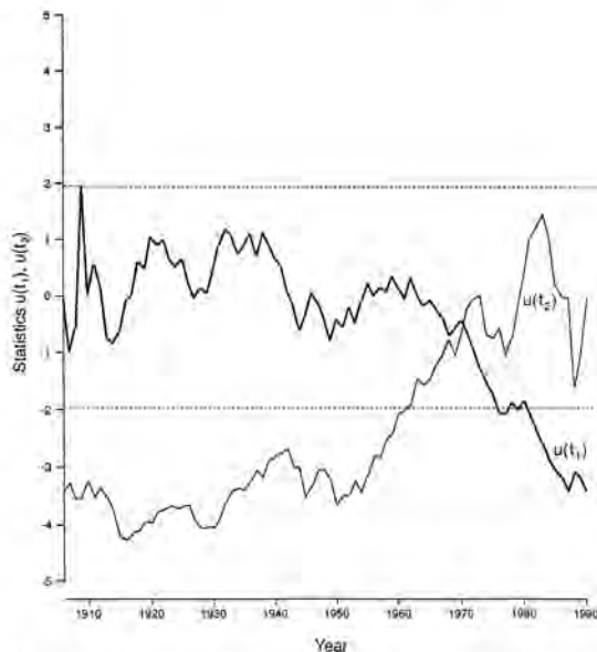
Fig. 3: Abrupt climatic change of the annual rainfall time series of Kano as derived from the sequential version of the Mann-Kendall-Sneyers test. u(t_1) and u(t_2) are direct and backward curves respectively.
