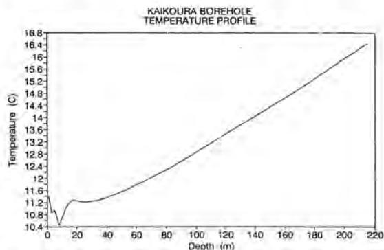
Fig. 2. The measured temperature-depth profile for the Kaikoura borehole.
