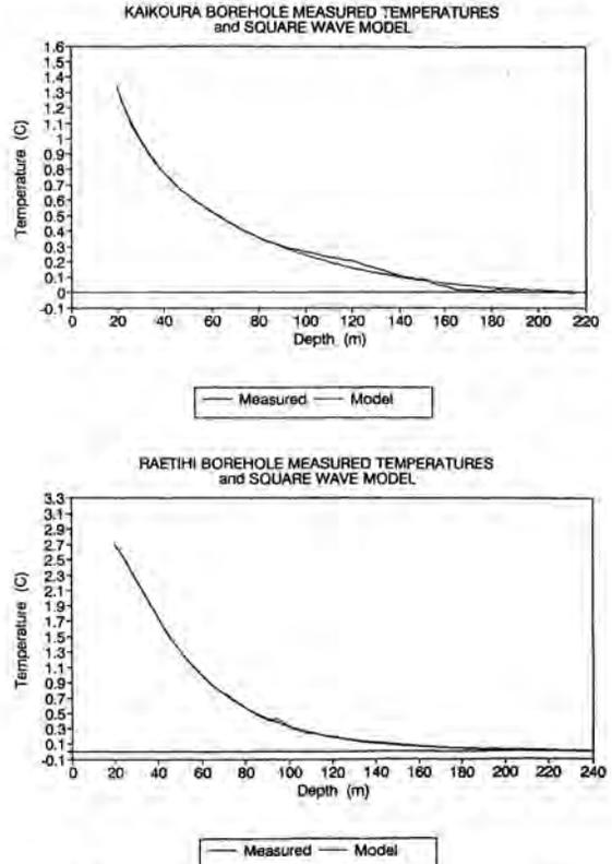
Fig. 5: The measured and theoretical temperature differences versus depth for the Kaikoura and Raetihi boreholes. The theoretical temperature differences are calculated from the model of surface temperatures consisting of a series of square waves.
