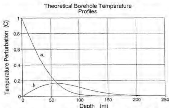
Fig. 1. The theoretical temperature-depth profiles for (a) a step increase in surface temperature of  $1^{\circ}\text{C}$  occurring 30 years ago, and (b) a square wave change in surface temperature of  $1^{\circ}\text{C}$  which began 80 years ago and finished 40 years ago.
