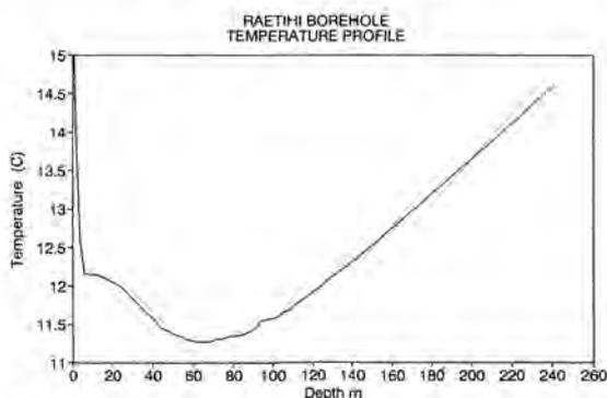
Fig. 3. The measured temperature-depth profile for the Raetihi borehole.
