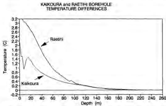
Fig. 4: The temperature differences versus depth obtained after removal of the geothermal gradient from the measured temperature-depth profiles for both the Kaikoura and Raetihi boreholes.
